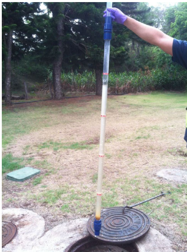
Figure 3-1: Sludge and Scum Measurements Taken with Sludge Judge
