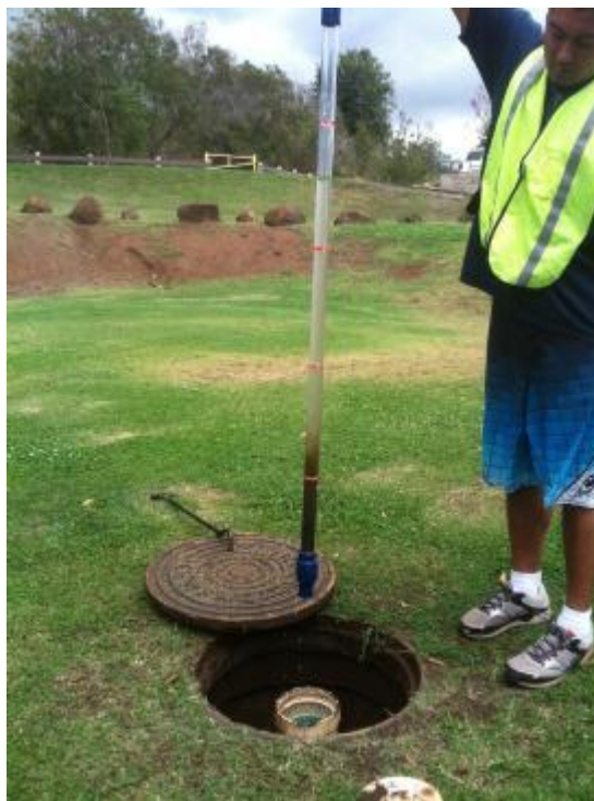
Fig. 17 Estimated sludge level of approximately 15 inches. No presence of scum for this water sample
