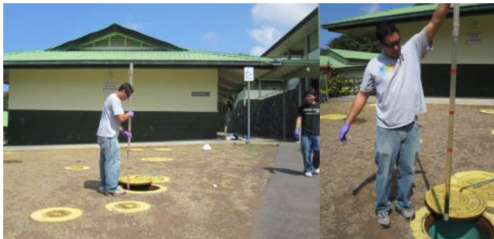
Fig. 14 and 15, Sludge and scum test being conducted on a septic tank.
