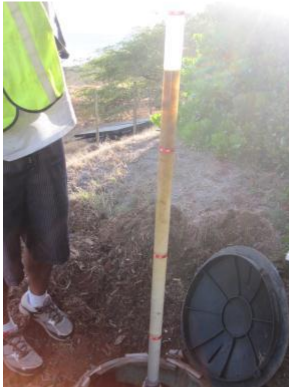
Fig. 16, Estimated scum level of approximately 10 inches. No presence of sludge for this water sample.
