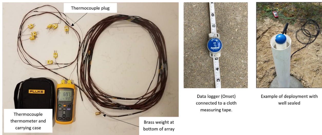
Figure 1: Examples of temperature arrays and deployment in field.
