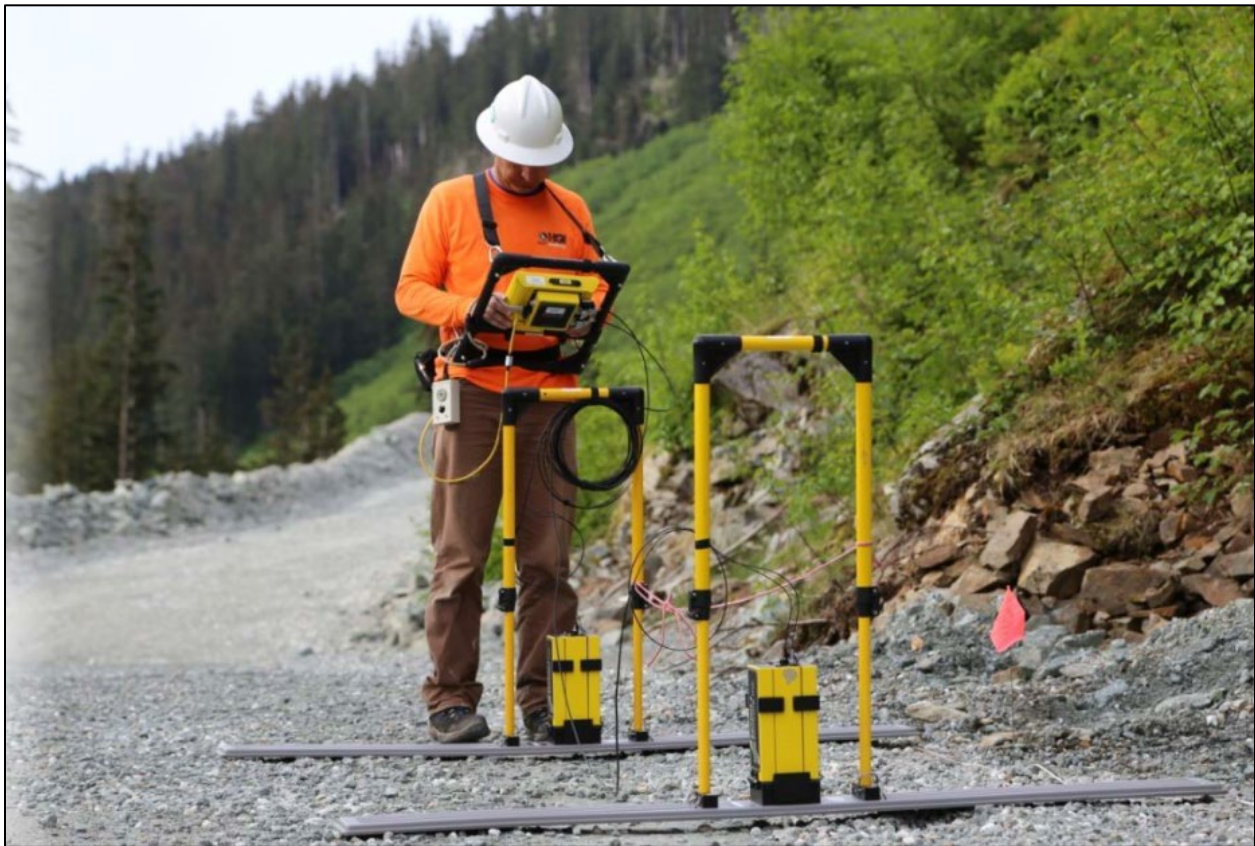
Figure 5: GPR pulseEKKO PRO System, with 50-MHz Antennae Frequency
