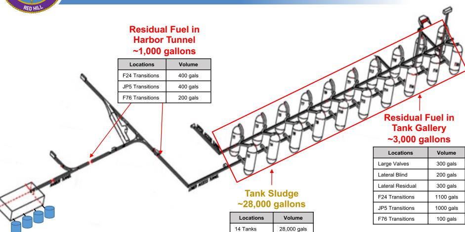
During Closure NCTF-RH will be responsible for the removal of ~4K gallons of residual fuel and ~28K gallons of sludge
