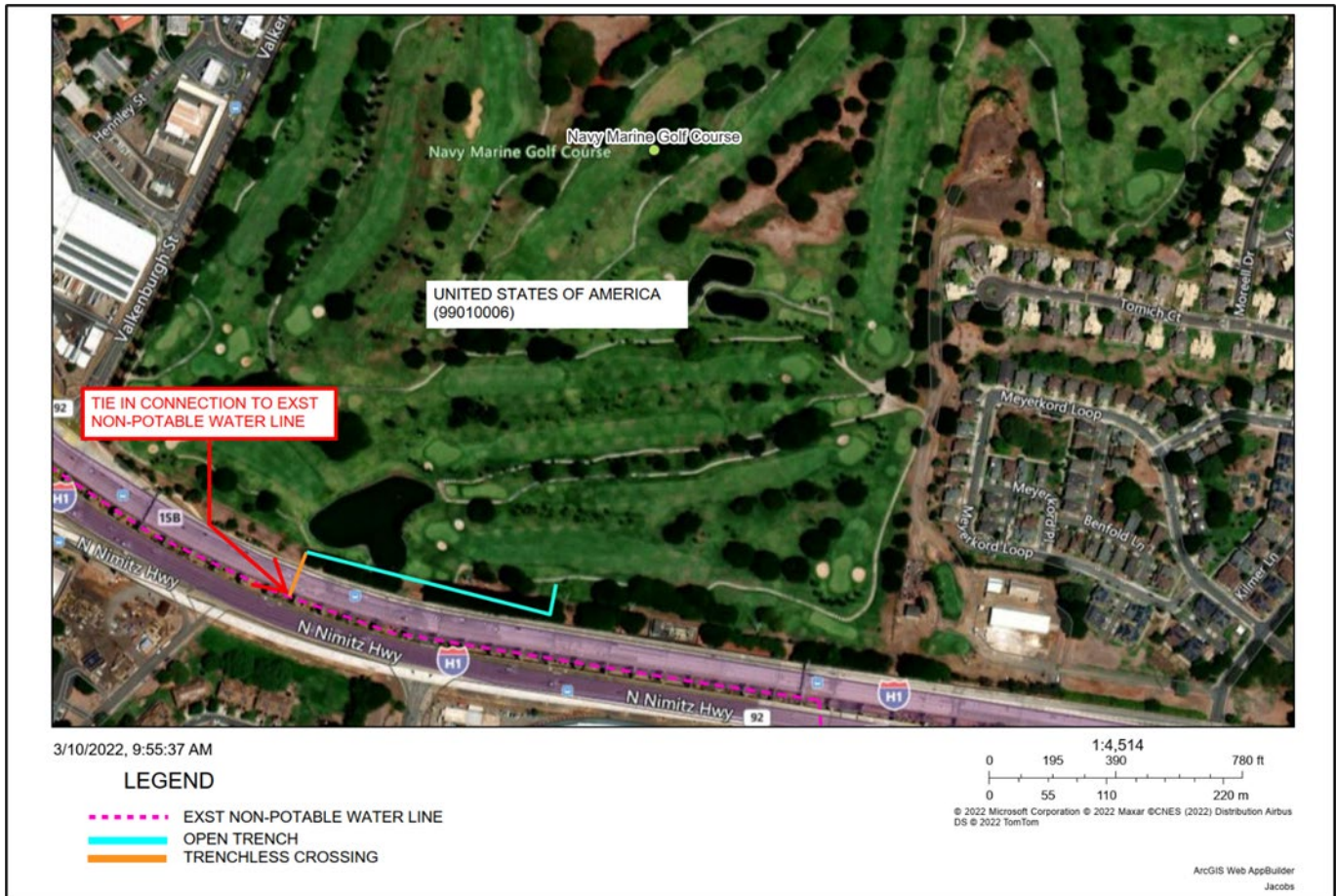
Figure 2-24. COA 4 Main Pond Buried Pipelines Map
