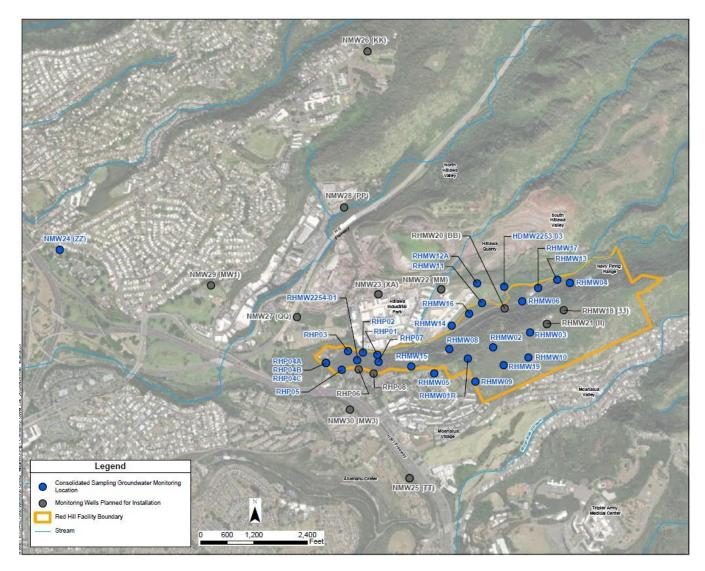
Figure 1. Groundwater Monitoring Well Sampling Locations.
