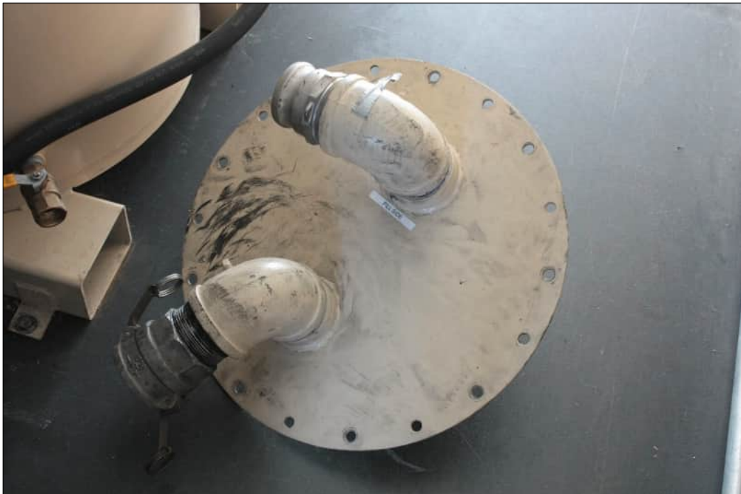
Photo 3. Manway adapter used to fill vessels with fresh GAC.
