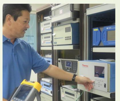
Installed Puna H monitoring station for ambient air pollutants
