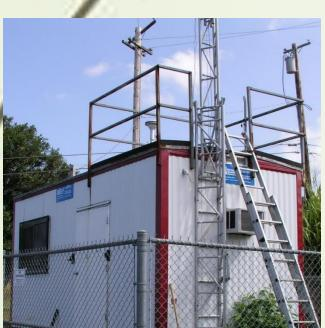
Installed Kona monitoring station for ambient air pollutants
