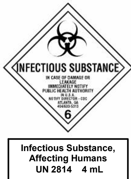
FIGURE 2 Labels which indicate an infectious substance (Class 6), proper shipping name, UN number, and quantity of substance.
