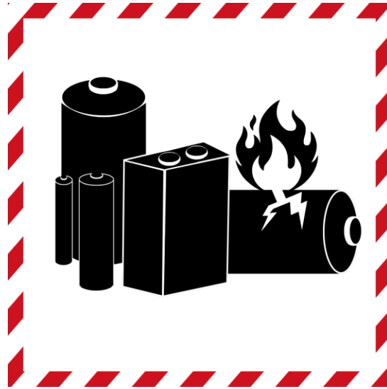
Image 1: Lithium-ion battery shipping label used for packages containing Lithium-ion batteries. Diagram of batteries in the middle and red border with white hatch marks around the label.
