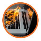
Thermal runaway, leading to a lithium-ion battery involved fire can be detected with a **loud pop and hissing noise** followed by a large amount of **initially white smoke** quickly followed by **dark smoke** that is highly **toxic and flammable. The smoke can ignite within seconds.**
