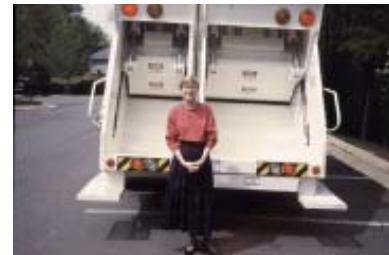
Photo 5-4. Rear-loader with two compaction units
