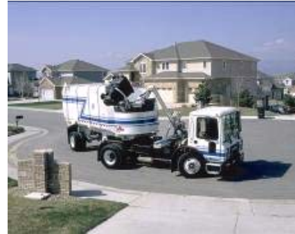
Photo 5-2. Heil's trailer collection vehicle that allows for tight turns and large loads
