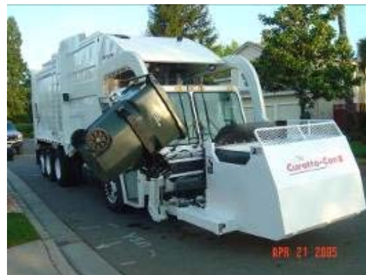
Photo 5-6. Front-end loader with a Curotto Can on the front for residential collection
