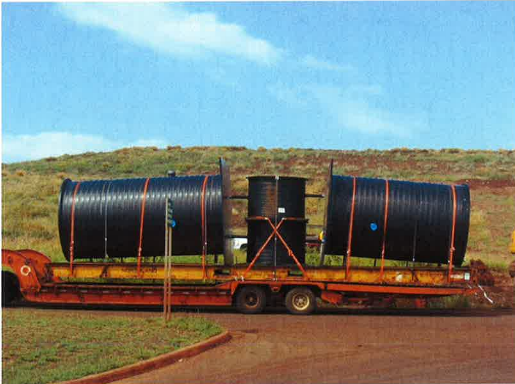
Photo 1. Wet well and meter valve box assemblies.
