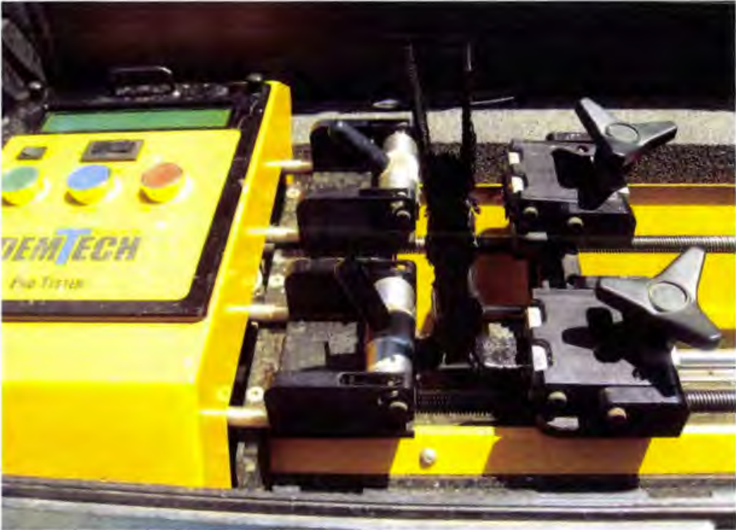
Photo 87. Field testing a trial seam for peel strength (textured geomembrane-to-flatstock extrusion trial weld shown above)
