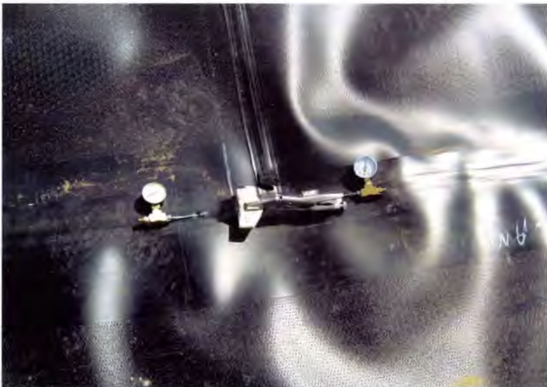
Photo 92. Non-destructive air pressure tests are performed for all double-fusion welded production seams (30 psi minimum held for 2 minutes)
