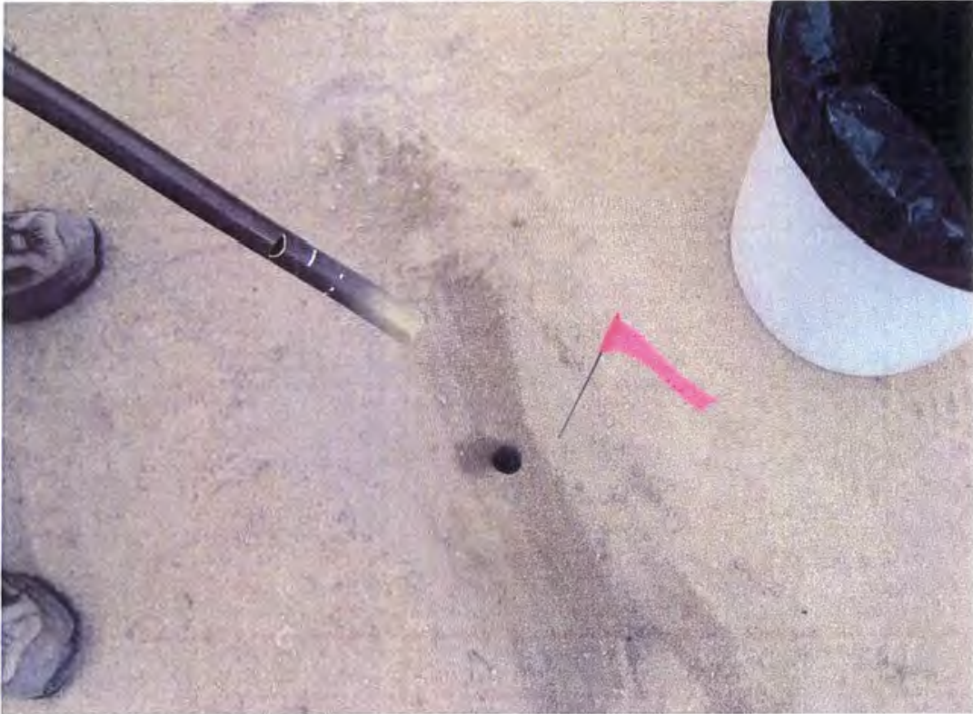
Photo 9. Samples were collected using a hollow metal rod, approximately 1-inch in diameter
