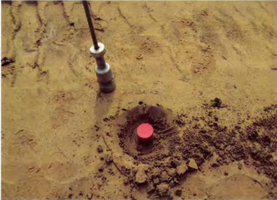
Photo 13. Collecting thin-wall Shelby tube samples for moisture-density determination by the drive cylinder method (ASTM D2937)
