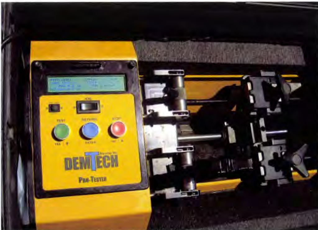
Photo 86. DemTech's Pro-Tester T-0100 tensiometer is used to field test the peel and shear of the trial welds
