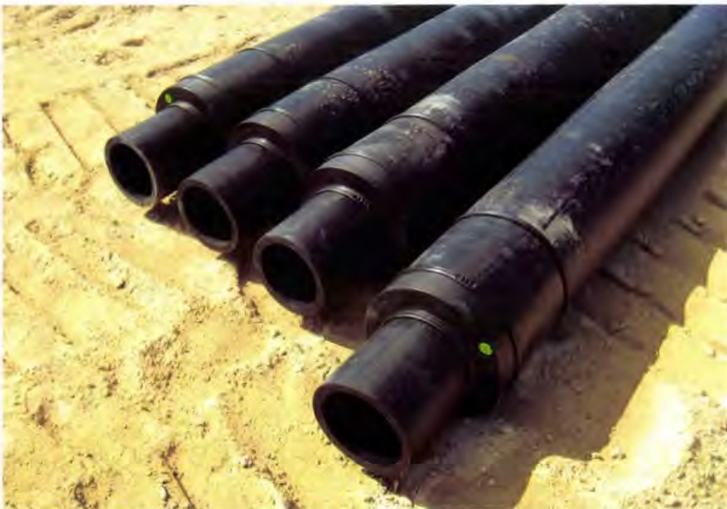
Photo 28. New dual containment, 4-inch diameter SDR 11 inside 8-inch diameter SDR 17 (4" \phi x 8" \phi ), HDPE pipe sections
