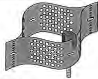
Figure 8 ATRA Anchor Connected Over the Cell Wall
