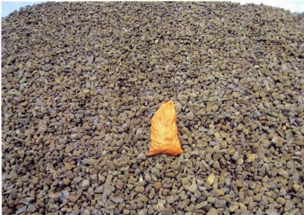
Photo 72. Collecting a sample of 3-inch minus granular fill material (imported from Kauai Aggregate Quarry) for conformance testing
