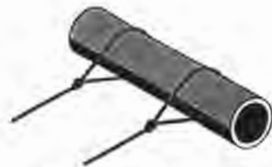
Figure 10 Tendon Secured to Deadman Anchor
