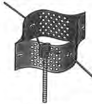
Figure 9 ATRA Anchor and tendon anchoring
