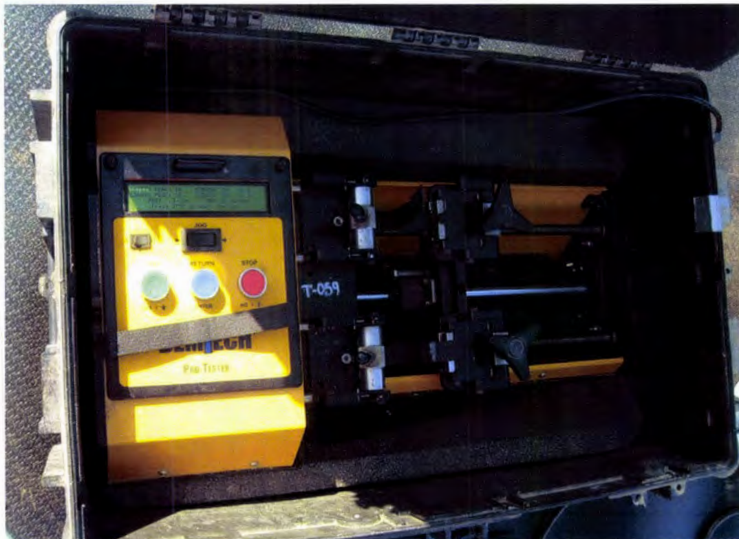
Photo 28. DemTech's Pro-Tester T-0100 tensiometer is used to field test the peel and shear of the trial welds
