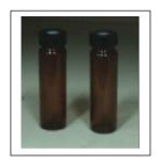
Fill out the sample labels and apply it to the sample vials. Remove any connections (hoses, etc..) from the sample tap. Flush the tap for at least 2-3 minutes and then fill both of the amber vials to the rim (forming a meniscus) with your water sample.
