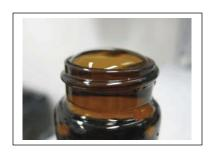
Place the caps on the vials being sure that the septa is teflon-lined side down (towards the sample). Avoid trapping air bubbles within the vials.
