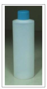
Fill out the sample label and apply it to the sample bottle. Remove any connections (hoses, etc..) from the sample tap. Flush the tap for at least 2-3 minutes and then rinse out the plastic bottle and the cap 3 times with the water you are sampling.
