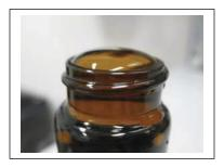
Place the cap on the vial being sure that the septa is teflon-lined side down (towards the sample). Avoid trapping air bubbles within the vials.
