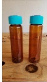
HERBICIDES - 2 - 40ml amber glass vials. Fill vials with water sample, create meniscus at top surface of water. Cap bottle. After capping, invert vial and check for air bubbles. If air bubbles present, repeat last step.
