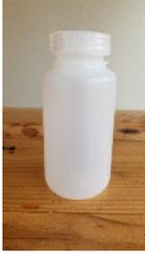
NITRATE - 1 - 250ml plastic bottle. No additives. Rinse bottle 3 times. Fill water sample to rim of bottle and cap bottle.
