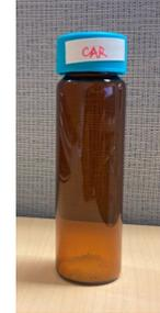
CARBAMATE - 1 - 40ml clear glass vial that contains a powdered preservative. Fill vials with water sample, create meniscus at top surface of water and cap vial. After capping, invert vial again and check for air bubbles. If air bubbles present, repeat last step.
