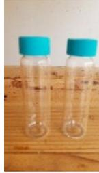
EDB/DBCP/TCP - 2 - 40ml clear glass vials. Fill vials with water sample, create meniscus at top surface of water. Cap bottle. After capping, invert vial and check for air bubbles. If air bubbles present, repeat last step.
