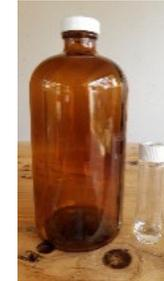
SOC - 1 - 1 L amber glass bottle. Fill bottle  $\frac{3}{4}$  full with water sample. Cap bottle and gently invert the bottle to mix water. Pour HCL from 40 ml clear glass vial into sample water. Fill bottle with water to the base of the neck and cap.
