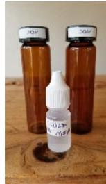
VOC - 2 - 40ml amber glass vials. Fill vials with water sample, create meniscus at top surface of water. Add 2 drops of HCL into sample and cap. After capping, invert vial again and check for air bubbles. If air bubbles present, repeat last step.
