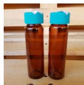
TRIHALOMETHANES- 2 - 40ml glass amber vials. Fill vials with water sample, create meniscus at top surface of water. Cap bottle without trapping air bubbles. After capping, invert vial and check for air bubbles. If air bubbles present, repeat last step.
