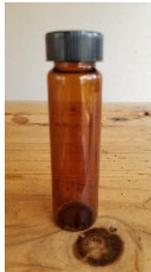
GLYPHOSATE - 1 - 40ml amber glass vials. Fill vials with water sample, create meniscus at top surface of water. Cap bottle. After capping, invert vial and check for air bubbles. If air bubbles present, repeat last step.
