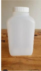
METAL - 1 - 500ml plastic bottle. No additives. Fill water sample to rim of bottle and cap bottle.
