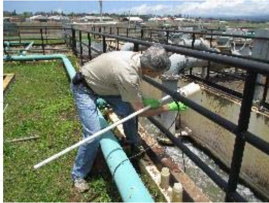
Wastewater & Reclaimed wastewater sampling for pharmaceutical & personal care products (PPCPs).
