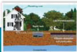
Figure 2. Cross-section of septic system with a soil absorption field.
