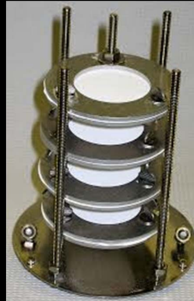
Membrane discs inside sampler absorb pesticides
