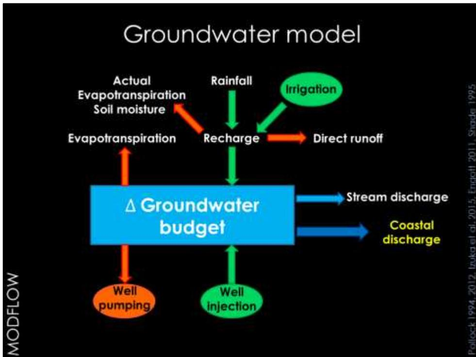
We parameterized the GW flow model (MODFLOW) based on what comes out of the aquifer, in terms of ET and pumping
