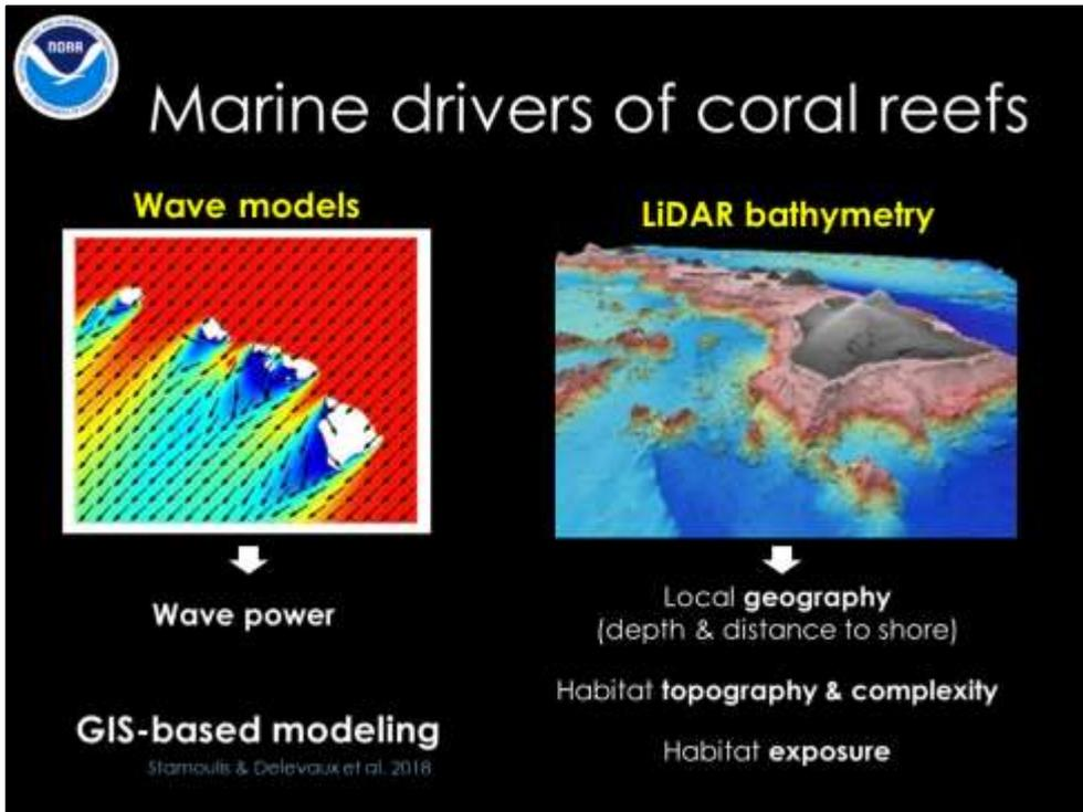
We used the SWAN wave model to derive wave power at both sites
