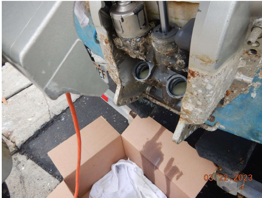
Photograph 11: View of fluid actively dripping from boat stored in maintenance area without containment. Photograph taken March 22, 2023 by Bobbie Teixeira.
