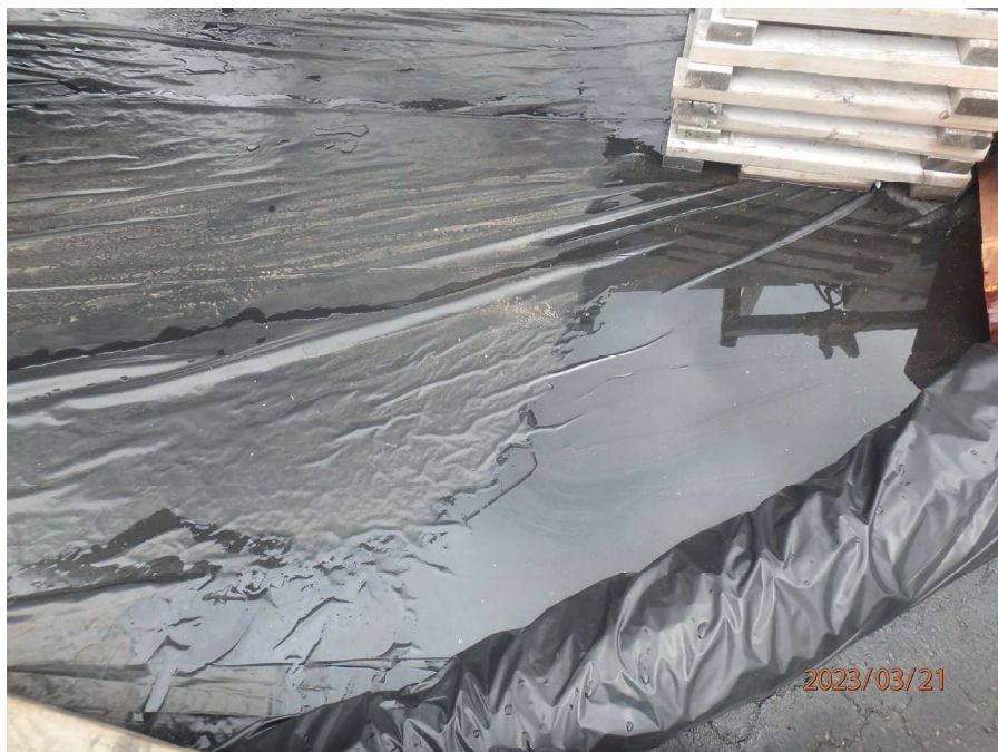
Photograph 7: Close-up view of sheen on surface of water accumulated within the containment for boat stored in the maintenance area. Photograph taken March 22, 2023 by Jacquelyn Corpus.
