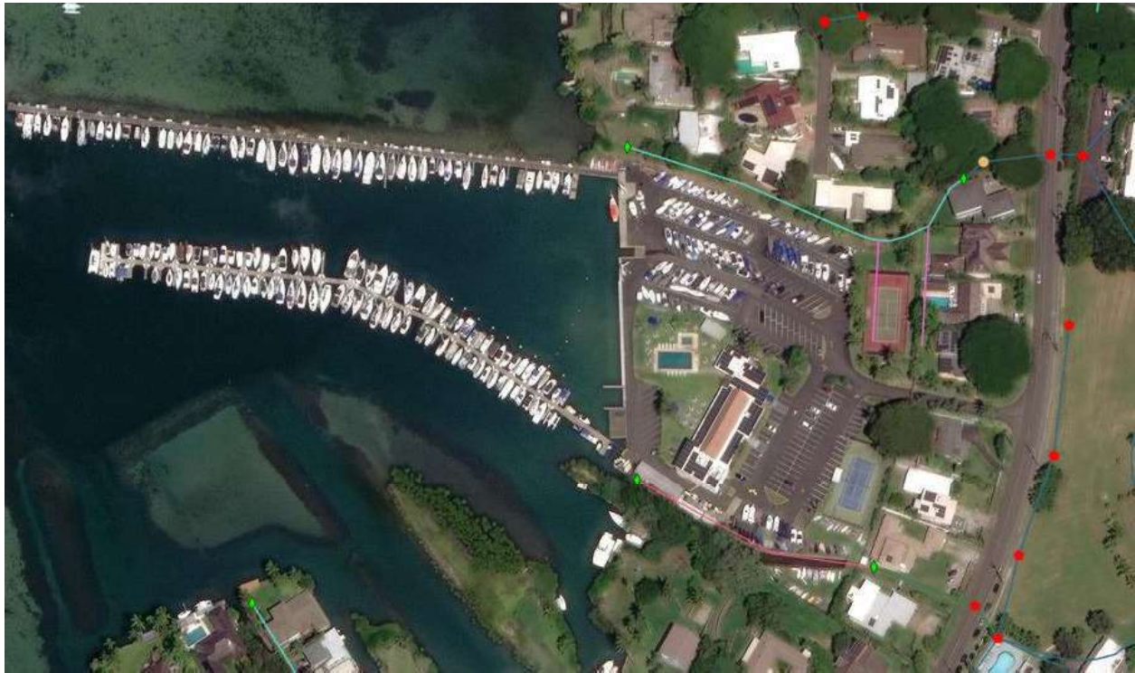
Image 1: Image of the Facility pulled from the Department of Transportation Highways Asset Management System. The image indicates the location of the CCH drainage system to Kaneohe Bay.
