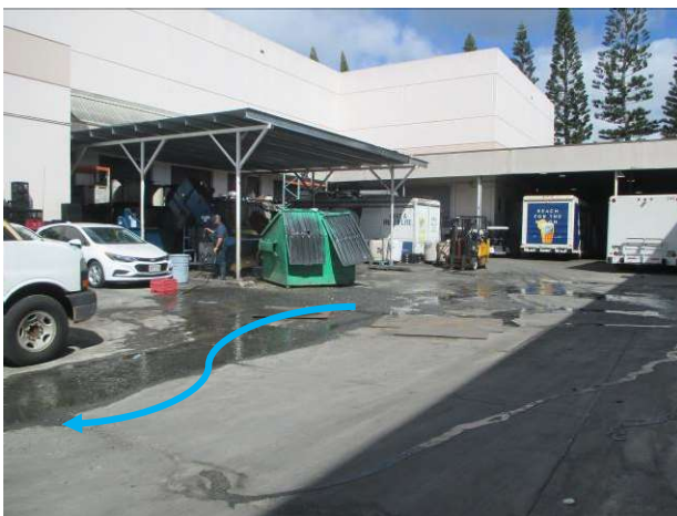
TMK: 9-4-128:002: A dry weather flow with an alcohol odor was observed flowing on the paved lot. The flow originates from the reclamation area where pallets of alcoholic seltzer water were sprayed down. (IMG_007)
