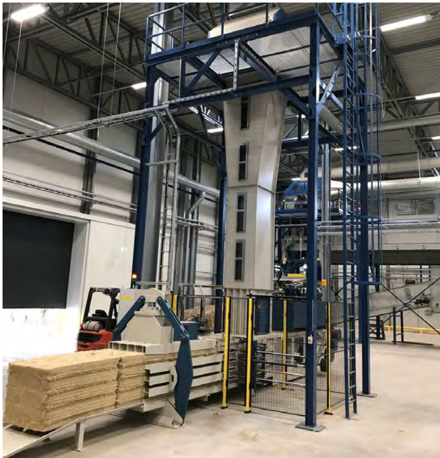
Automatic fiber baler fed by an air separator
