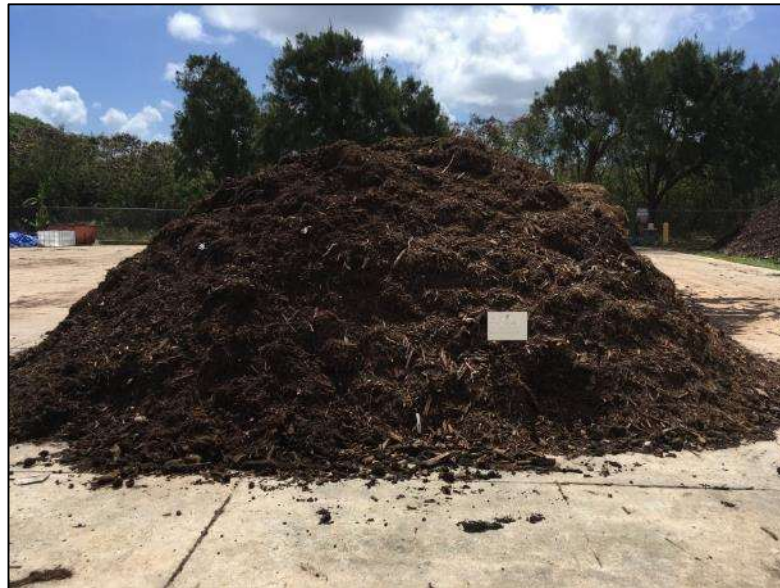
Figure 4. Stockpile of compost prepared of a 3:1 mixture of green waste and biosolids at WWTP #6 (used for on-site landscaping).
