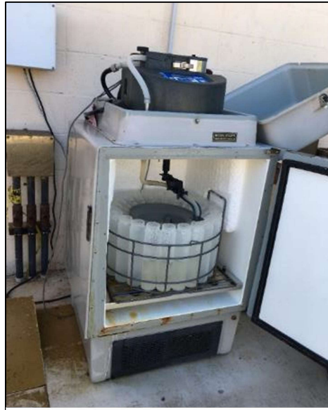
Figure 8. Composite sampler equipment used to collect 24-hour samples of influent and effluent at wastewater treatment plants.
