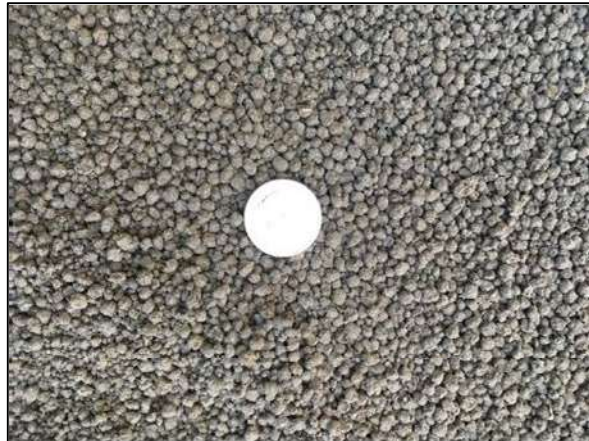
Figure 9. Pellets of dried biosolids used as fertilizer on golf courses and landscaped areas.
