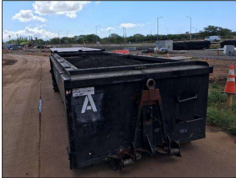
Figure 3. Twenty cubic yard roll-off bins used to collect and transport biosolids at wastewater treatment plants.
