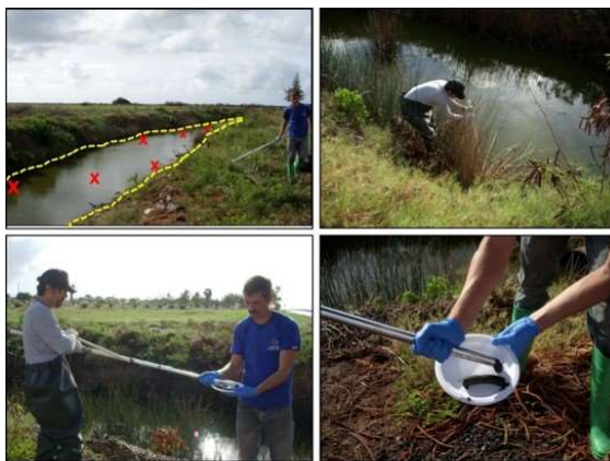
Figure 3-19. Use of a simple tube attached to piping to collect sediment sample increments in a shallow canal.
