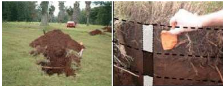
Figure 3-13. Use of exploratory pits, trenches and borings for initial investigation of subsurface soil contamination and exposure of DU layers for more detailed testing.
