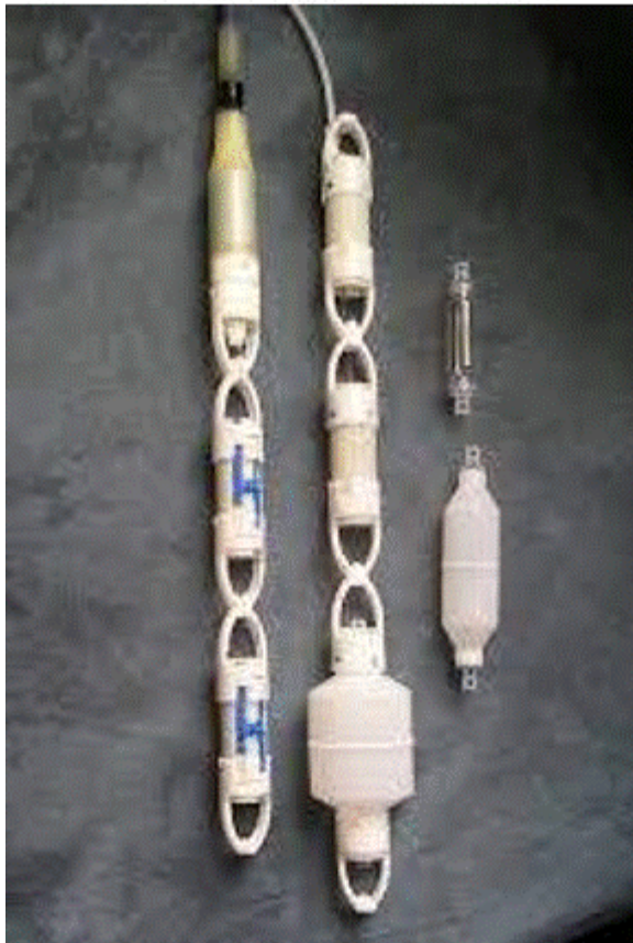
Figure 6-27. Snap Sampler passive sampler device. Top: Sampler bottle and holder device. Bottom: Series of Snap Samplers configured for deployment in a well.
