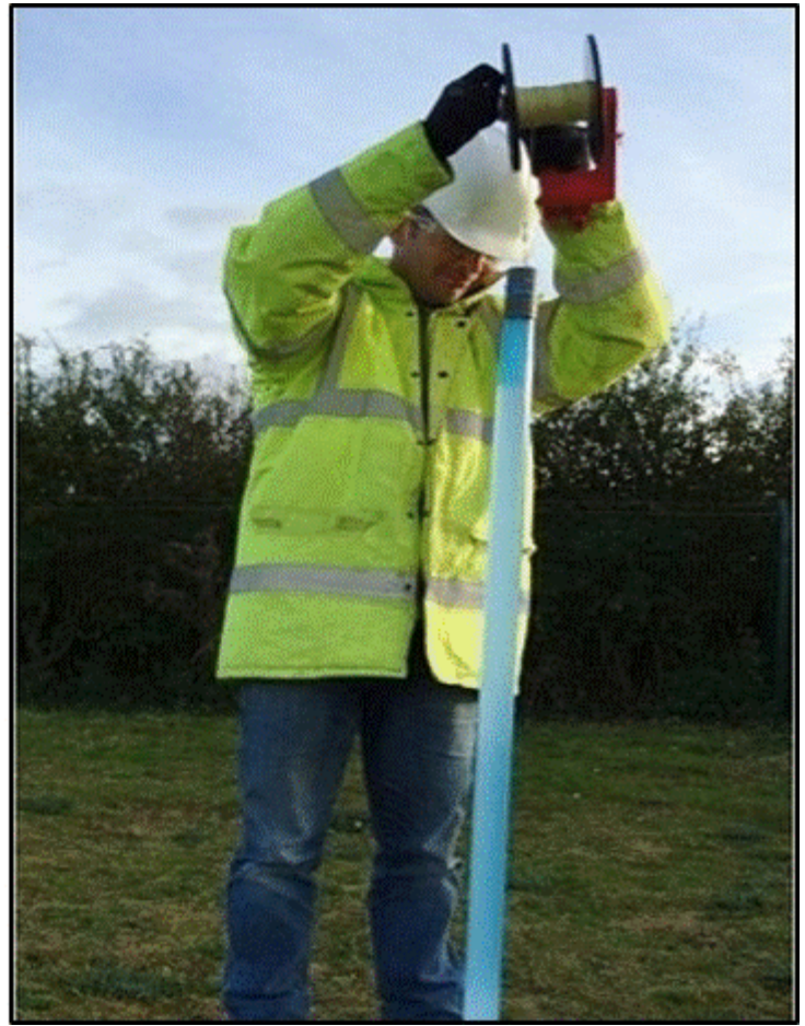
Figure 6-28. HydraSleeve before and after filling.
