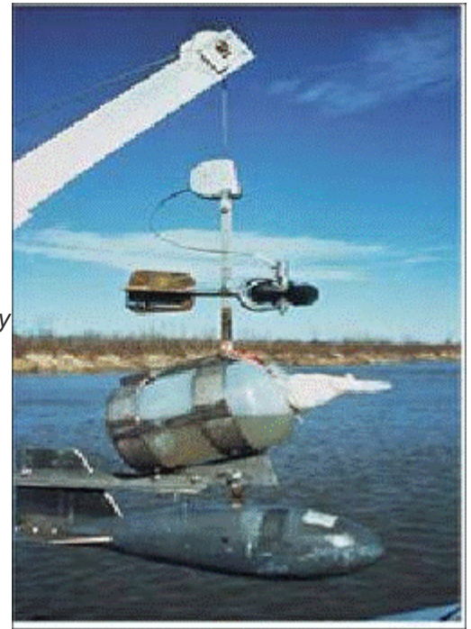
Figure 6-8 Isokinetic Sampler Constructed of Teflon. [Source: USGS, 2008b ]
