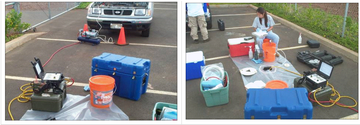
Figure 6-24. Field Setup for Purging and Sampling Well
