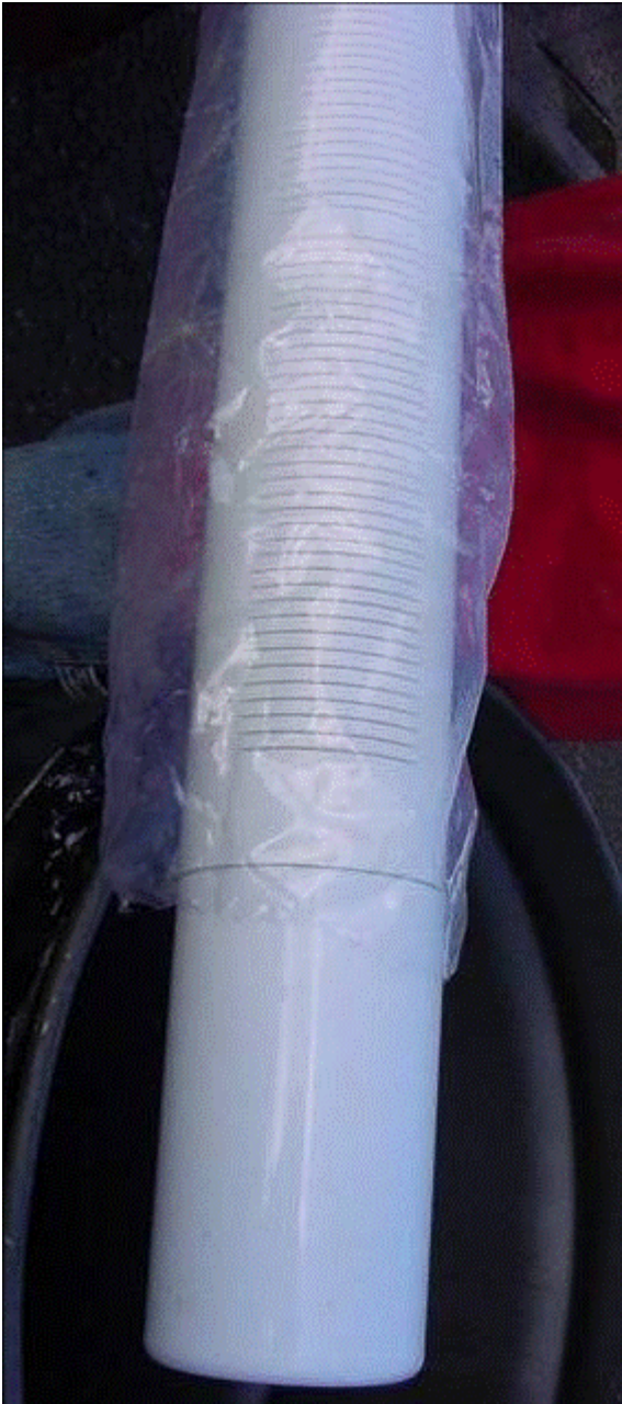
Figure 6-14. Portion of PVC Well Screen and Flush Threaded Bottom Cap
