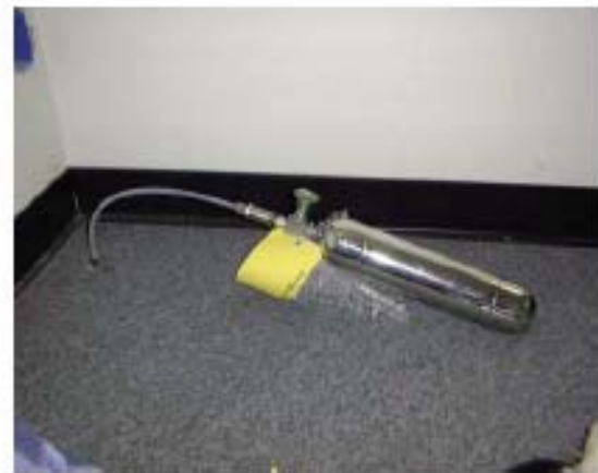
Figure 10. Sampling in 1-L evacuated canister for TO-15 analysis
