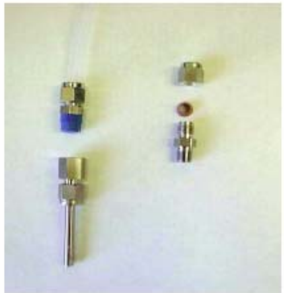
Figure 4. Stainless steel sub-slab vapor probe components
