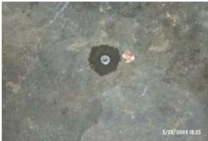
Figure 5. Completed vapor probe installation
