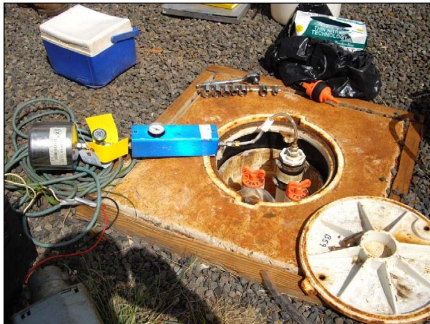
Figure 11. Connection of Summa and flow controller sampling train to vapor monitoring point.
