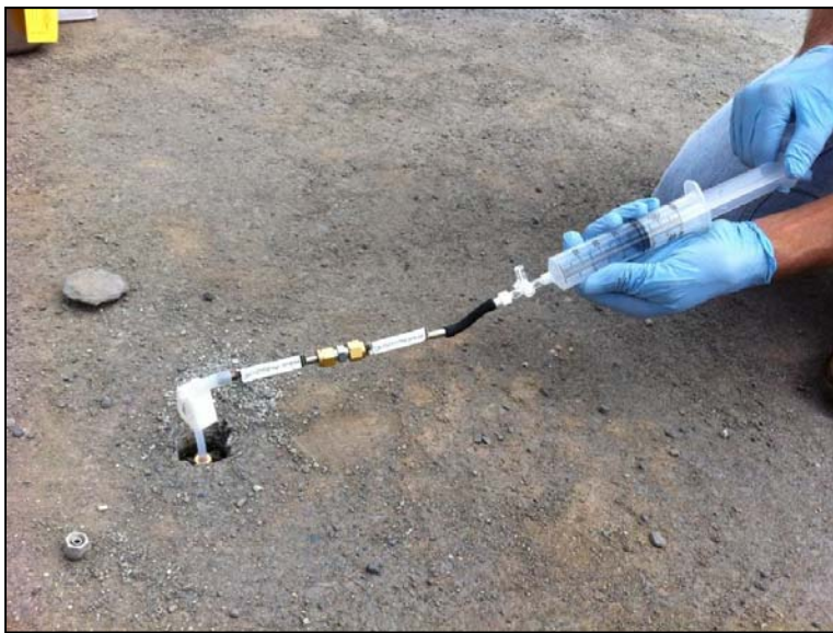
Figure 15. TO-17 sorbent tube sampling train using a 60ml syringe (50ml draw over thirty seconds for maximum 100 ml/minute flow rate; note use of second/upstream tube to check for breakthrough).
