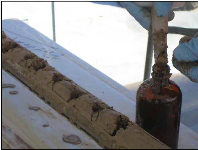
Figure 9. Preparation of core increment samples by subsampling targeted DU layer intervals.
