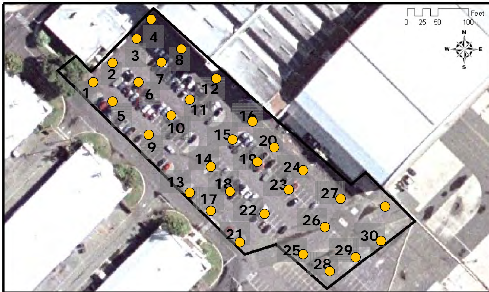
Figure 6. HDOH study DU borehole locations (approximate 70-foot grid).
