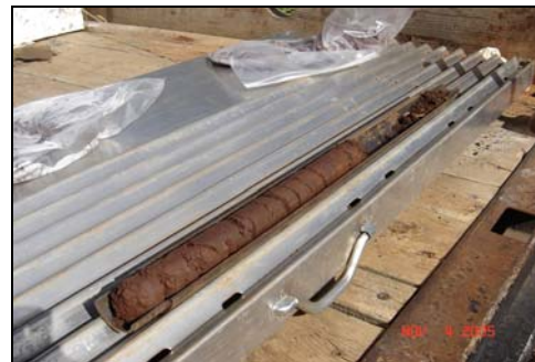
l) Continuous core collected from boring. The core represents an "increment" collected the subsurface portion of the targeted DU soil (photo from Bureau Veritas).
