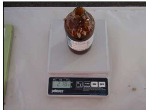
d) Total weight of plugs collected from increment monitored to ensure consistency between boreholes.
