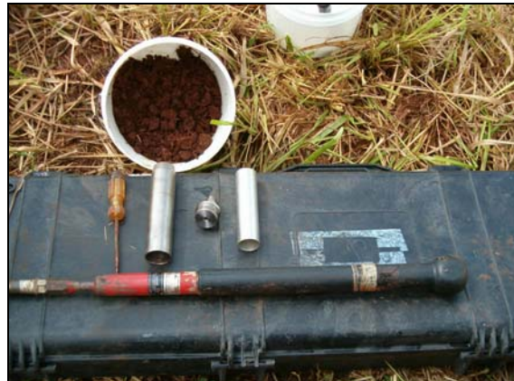
d) Core barrel removed and soil sample placed in field container (photo from Bureau Veritas).
