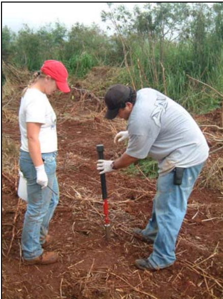
c) Use of a slide hammer to collect surface increments in hard soils.
