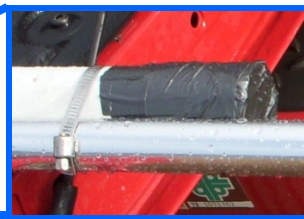
d) Sampling tube attached to bottom PVC piece with two metal hose clamps. Bottom piece of PVC sealed to keep mud & water out.
