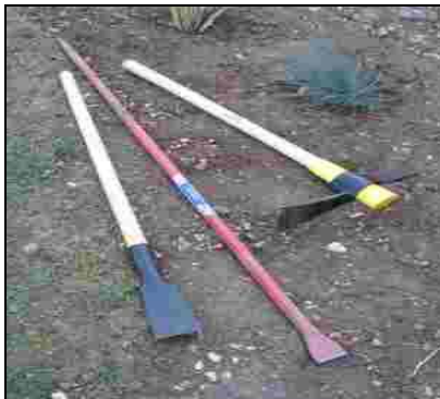
e) Narrow spade (root digger), o'o (pry bar) and mattock for collection of increments from hard-packed soil.
