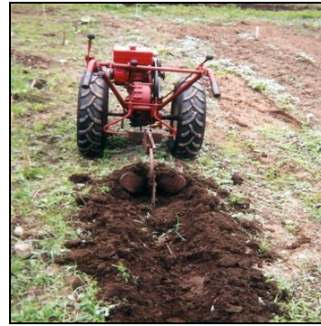
h) Cut furrows for collection of increments from hard-packed or gravelly surface soil.
