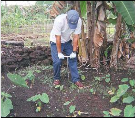
a) Use of an open-sided, sampling tube to collect surface increments in soft soils.
