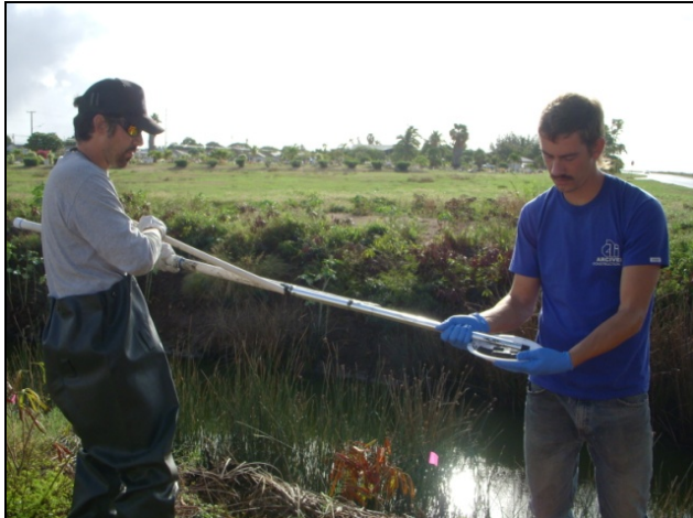
c) Increment core pushed out of tube using disposable 3/4" wooden dowel. Tilt tube slightly backward before pushing out sample in order to drain excess water, but be careful not to lose sediment.
