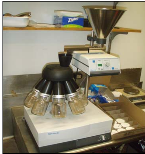
b) Subsampling of dried and sieved MI sample using a sectoral splitter.
