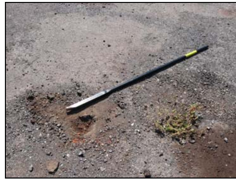
f) Breaker Bar used to cut through old asphalt surface and collect soil increments.
