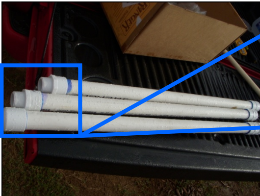
a) Ten-foot long PVC pipe for pole handle cut into five, 2' lengths for easy assembly in field (1" diameter Schedule 40) .
