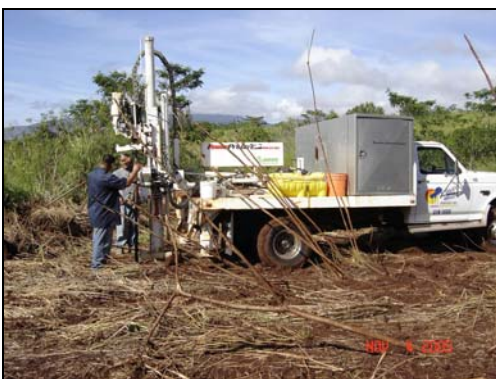
k) Push-drive rig used to collect subsurface soil increments (photo from Bureau Veritas).
