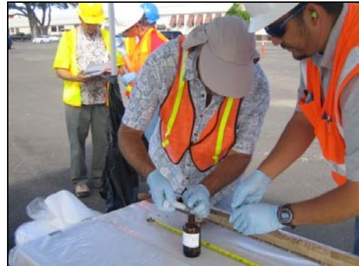
b) Core increment subsampled by collection of 5g plugs at regular spacing (e.g., every two inches).
