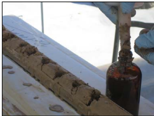
c) Plugs removed from DU Layer increment and placed in methanol.
