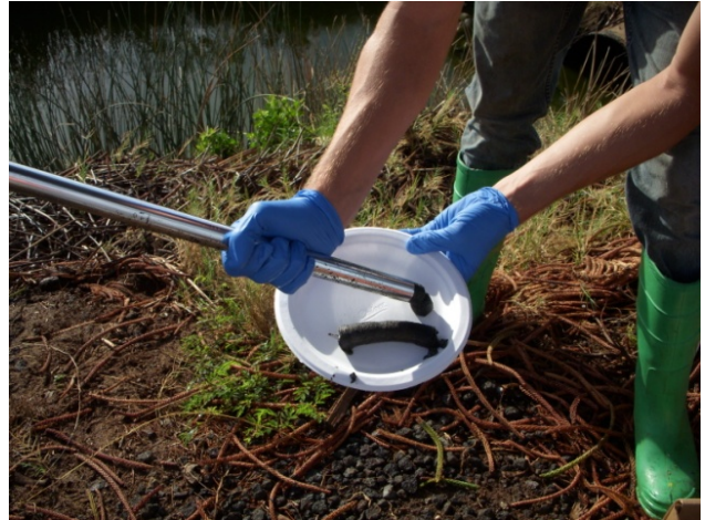
d) Increment collected on disposable plate and placed into sampling container (e.g., one-gallon freezer bag carried in clean bucket). Note cylindrical shape of increment.
