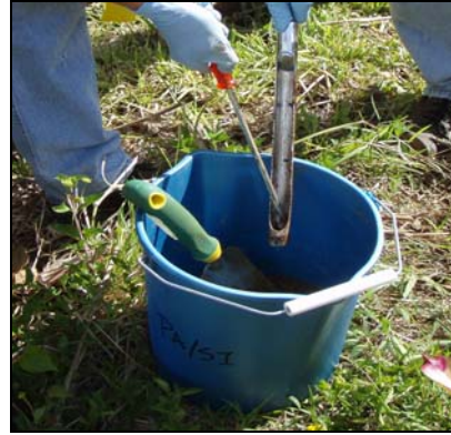
b) Use a flat-headed screwdriver to remove soil increment from tube.
