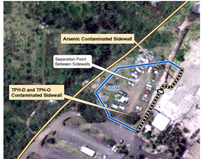
Example of map noting specific areas of contamination onsite as well as types of contamination.
