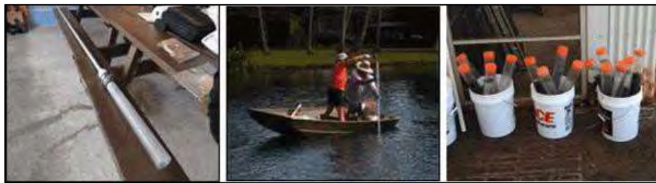
Figure 3-3. Use of core sampling tube to collect increments for the preparation of Multi Increment sediment samples. Left Photo: Core sampler attached to valve and push rod. Middle Photo: Manual collection of sediment core increment from skiff. Right Photo: Individual core increments collected from a sediment DU.
