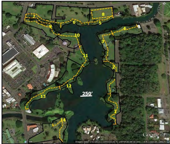
Figure 2-2. Soil Decision Unit areas tested as part of a 2013 Hawaii Department of Health investigation of arsenic in soil around the immediate perimeter of Waiakea Pond in Wailoa River State Recreation Area (HDOH 2013).
