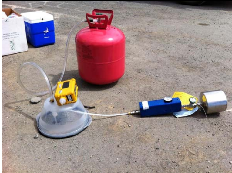
Figure 14. Use of a Tupperware container as a helium shroud during Phase II of the study (see also Attachment 4).
