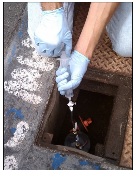
Figure 15. TO-17 sorbent tube sampling train using a 60ml syringe (50ml draw over thirty seconds for maximum 100 ml/minute flow rate; note use of second/upstream tube to check for breakthrough).
