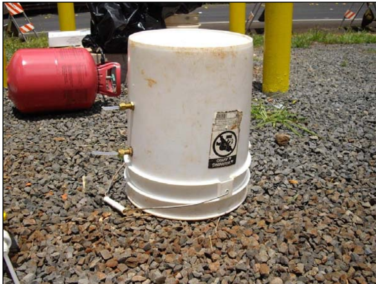
Figure 13. Five-gallon plastic bucket shroud with ports for sample collection and helium injection (not used due to height of the combined Summa canister and flow controller obtained from the lab for this study).
