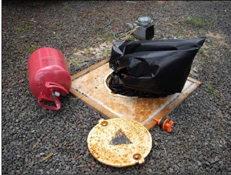
Figure 12. Use of a plastic garbage bag as a helium shroud during Phase I of the study.
