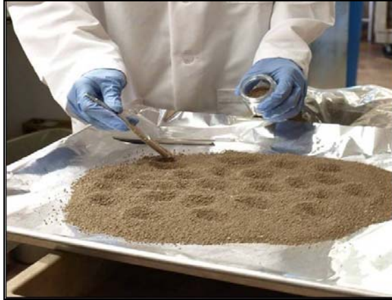
Figure 8-3. Collection of subsample for analysis from processed soil sample following drying and sieving in accordance with incremental sampling procedures.
