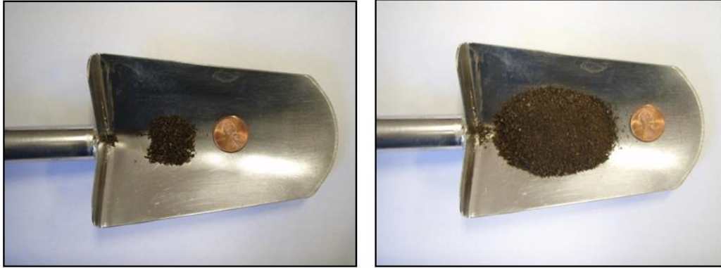
Figure 8-1. Size of soil subsample masses typically tested for metals (one gram, left photo) and PCBs (ten grams, right photo) by commercial laboratories (minimum ten grams recommended for metals in HDOH guidance; HDOH 2008).
