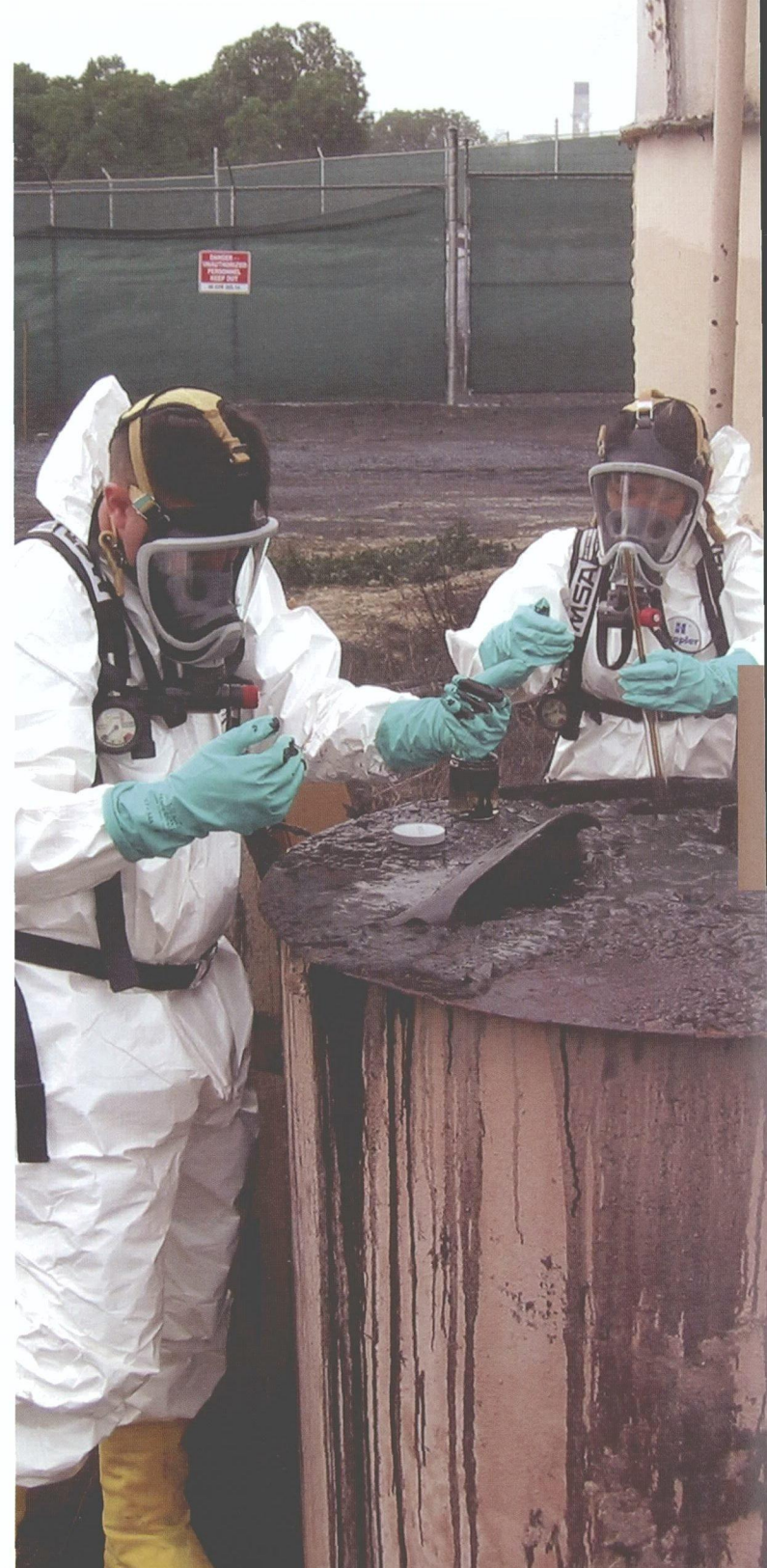
Cleanup workers taking samples at a leaking storage tank site. The first step in cleaning up sites like this is to assess what contaminants are present.
