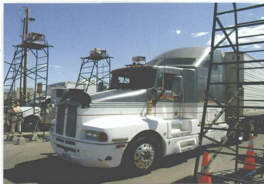
Monitoring system to measure air pollution from diesel trucks crossing the U.S.-Mexico border.
