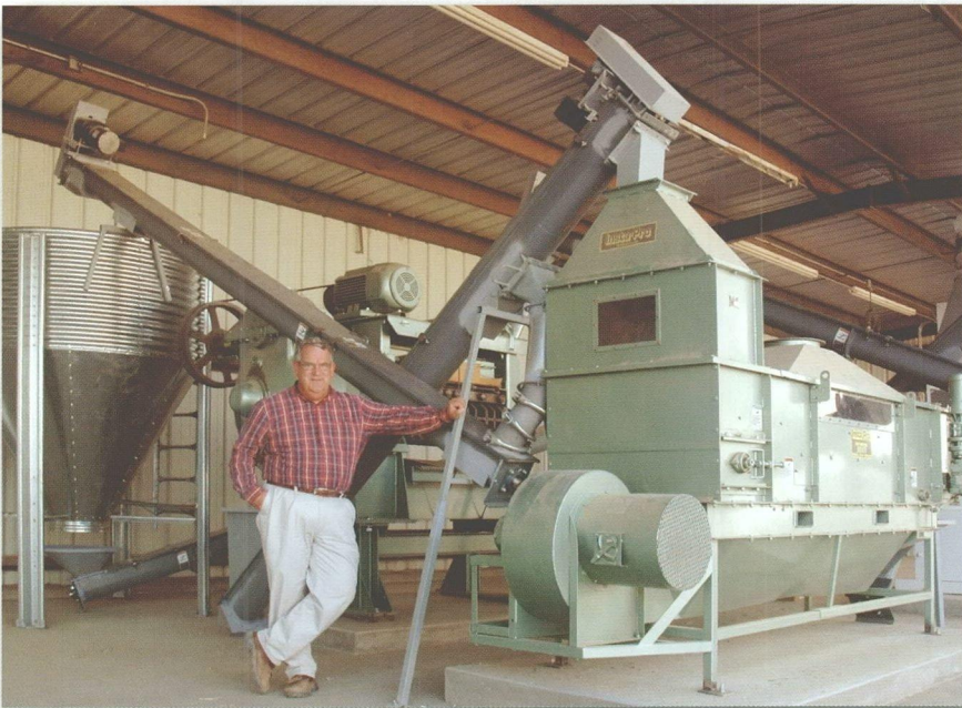
Top: Sunflowers at Red Rock Ranch near Fresno, Calif. Bottom: John Diener, owner of Red Rock Ranch, with oil press he uses to make biodiesel fuel from sunflower and safflower seeds.
