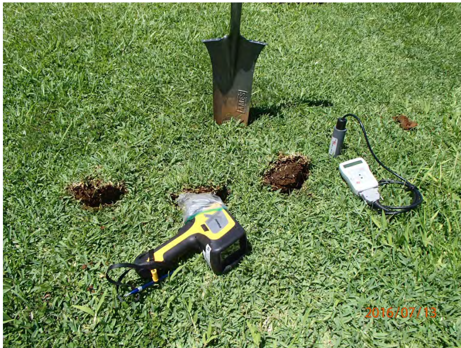
Photograph 2. XRF Analysis of Surface Soil, Performed in Triplicate, Soil Moisture Measured for XRF Value Correction (July 13, 2016)
