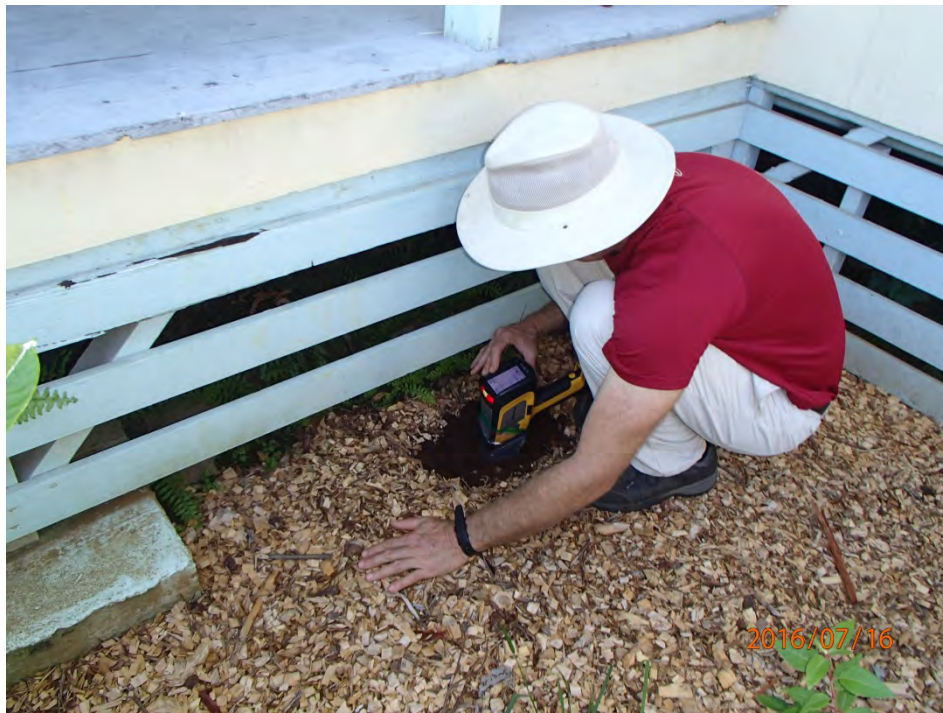
Photograph 4. XRF Analysis of Surface Soil along Building Perimeter, Keauakaha Elementary School (July 16, 2016)
