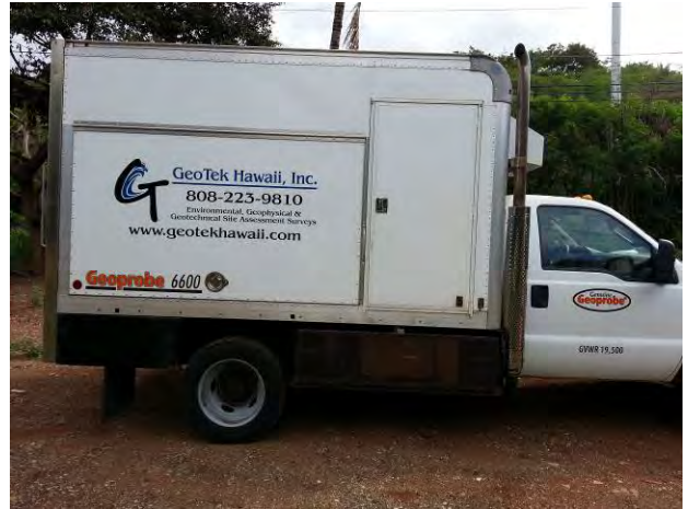
Photo 32. Truck-mounted drill rig used for drilling.
