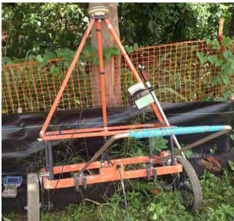
Photo 5. EM61 cart for geophysical survey.
