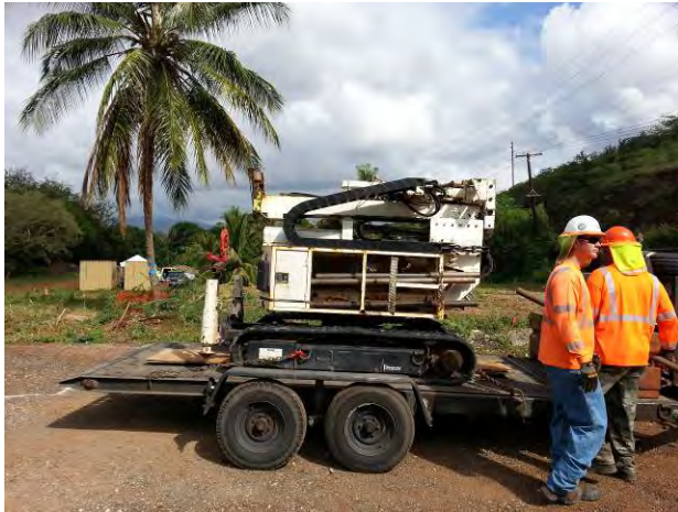
Photo 31. Track rig used for drilling.
