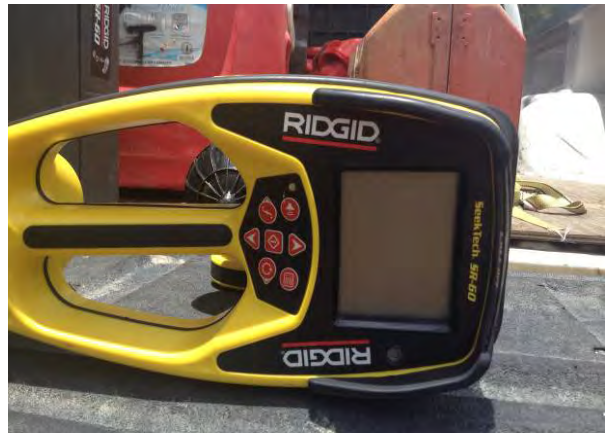
Photo 6. Ridgid Seek Tech SR-60 for utilities locating/clearing.
