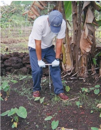
This picture shows soil sample collection from a small garden. Gardens grown near house foundations or near busy roadways have the potential for elevated soil lead concentrations.
