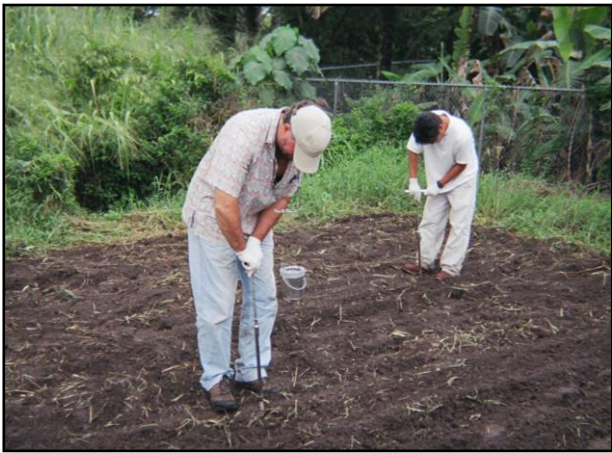
This picture shows soil sample collection from a small garden located on the island of Hawai'i. The garden is on former sugar cane land and therefore has the potential for elevated soil arsenic concentrations. Soil testing for arsenic will confirm if arsenic levels are elevated.
