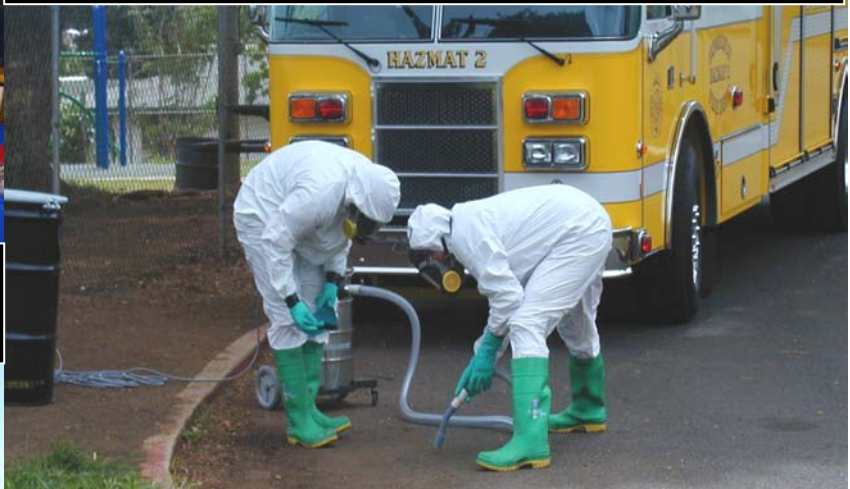
Hazardous Materials Response Team recovering spilled mercury droplets with a mercury vacuum
