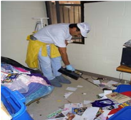
Screening a room for mercury vapor within the 260 units at Puuwai Momi Housing Complex
