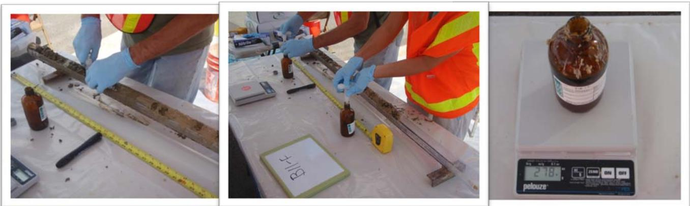
To collect a MIC sample, each core was sub-sampled by collecting multiple 5-gram increments of soil at a designated spacing interval using a Terra Core sampling device (Left). Each increment was transferred to an amber container filled with methanol to minimize loss of VOCs (Center). After all increments were collected, the weight of the MIC sample in the amber container was recorded (Right).
