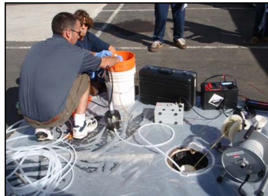
Above – A representative from Geotech Environmental Equipment demonstrates the use of a multi-probe field meter with flowcell. This instrument is used to measure water quality parameters while collecting samples directly from the well.
