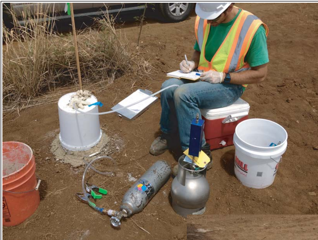
Photograph 5: Sample collection setup with helium cylinder in foreground next to Summa canister.
