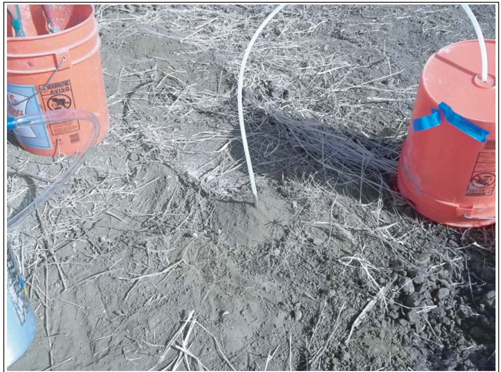
Photograph 2: View of tubing connected to soil vapor probe exiting ground surface.
