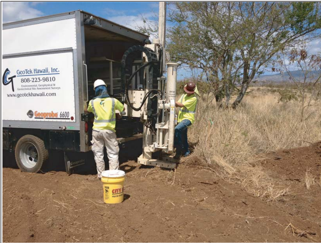
Photograph 1: GeoTek Hawaii installing soil vapor probe using direct push rig.
