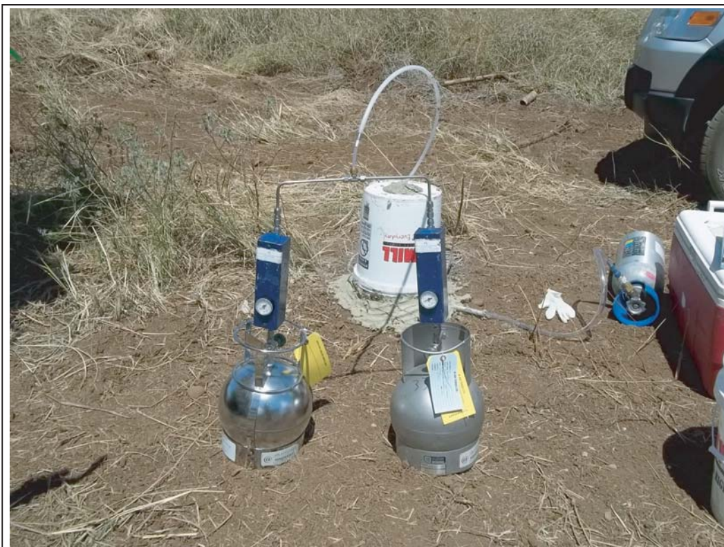
Photograph 4: Duplicate sample collection using "T" manifold to connect two Summa canisters.
