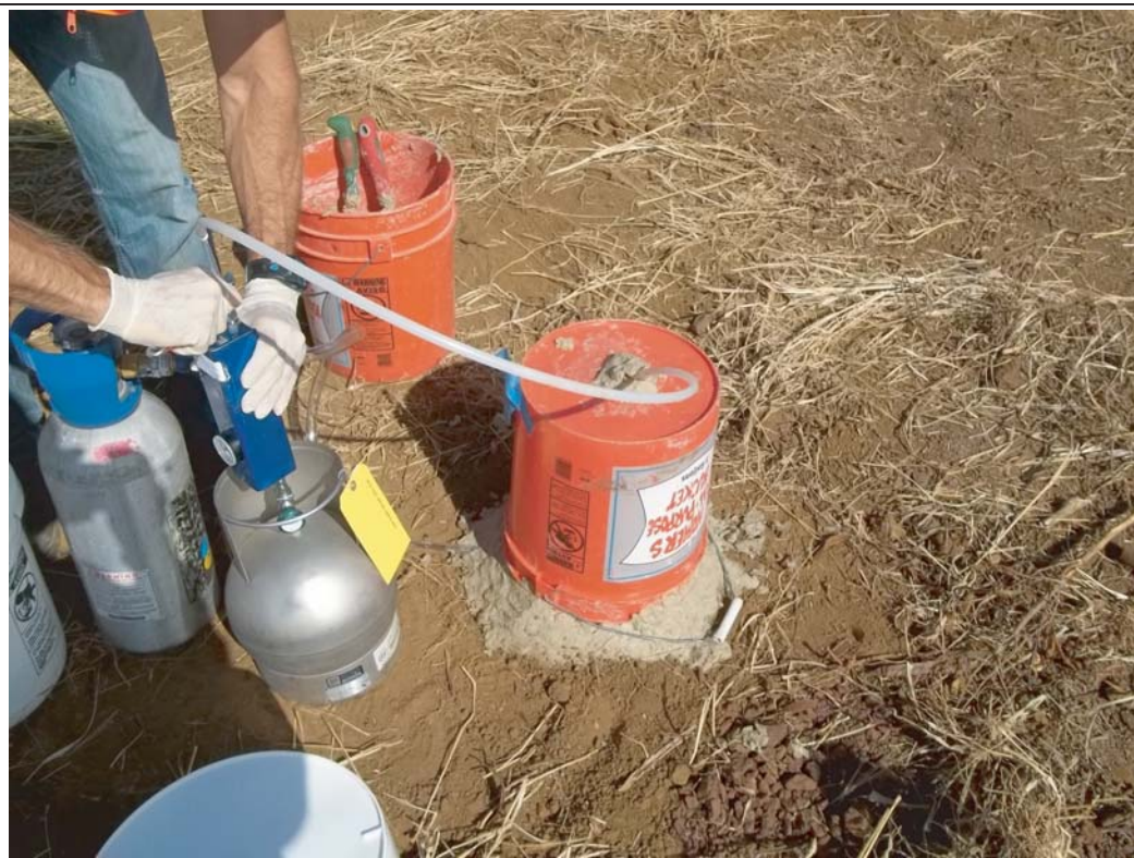
Photograph 3: Tubing from soil vapor probe being connected to flow controller and Summa canister.
