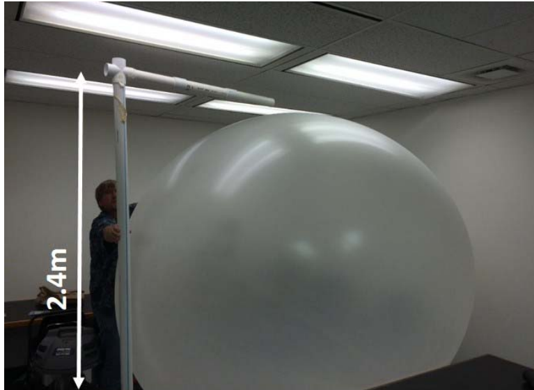
Figure 4-7. Latex, weather balloon used to check flow rate meters and evaluate purge times required to reach target, 7,000-liter purge volumes (target volume reached when balloon diameter = 2.4 m or 7.8 ft).
