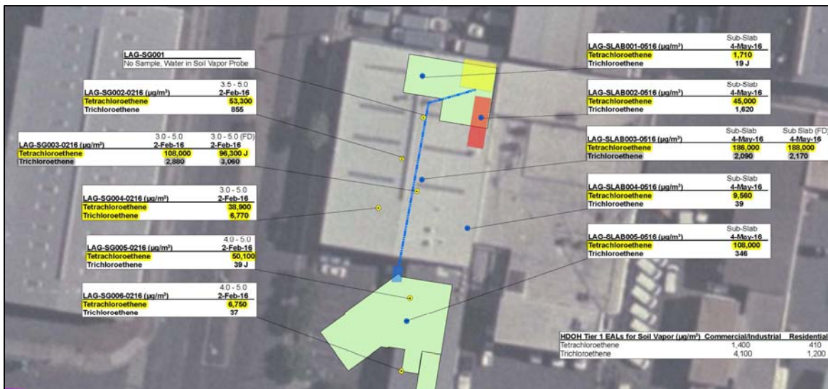
Figure 2-11. Summary of 2016 active soil gas data (CH2M 2017; preliminary data).
