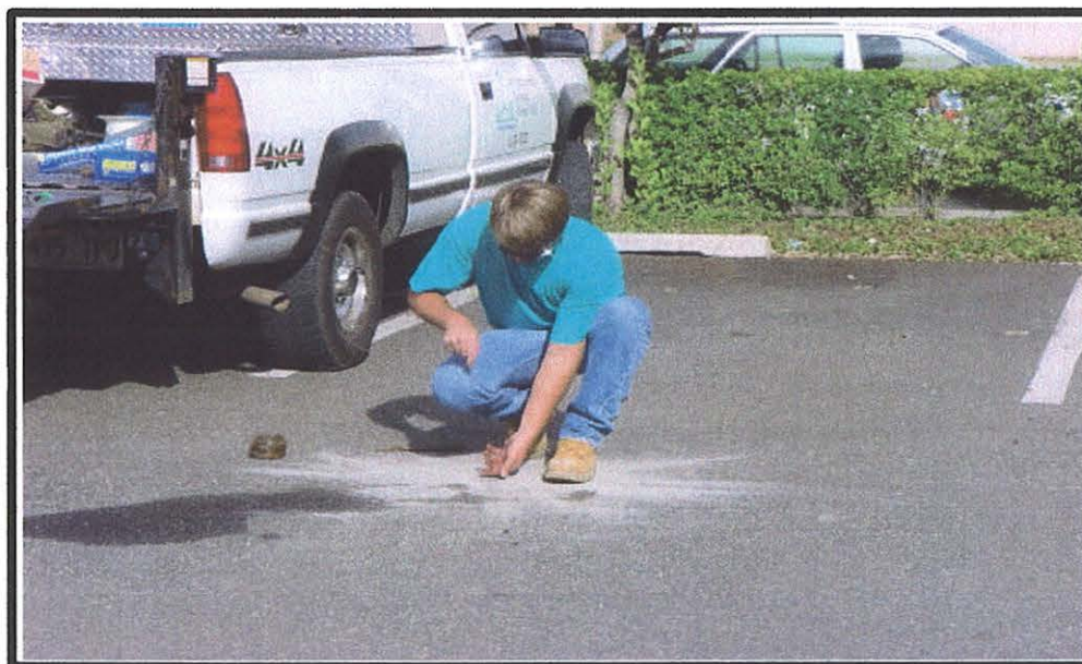
Photograph 2 : View of passive soil vapor module being installed.
