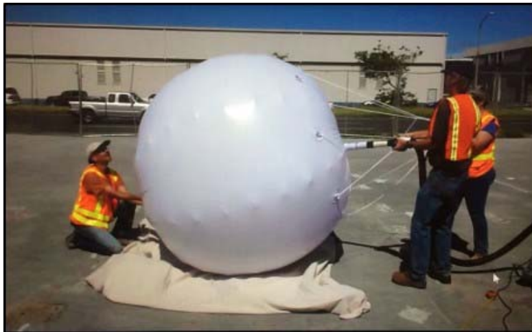
Figure 4-12. Weather balloon (vinyl) field test used to cross-check the purge volumes estimated from by flow rate meters; comparison of balloon volume to flow rate measurements and purge time indicated good correlation.
