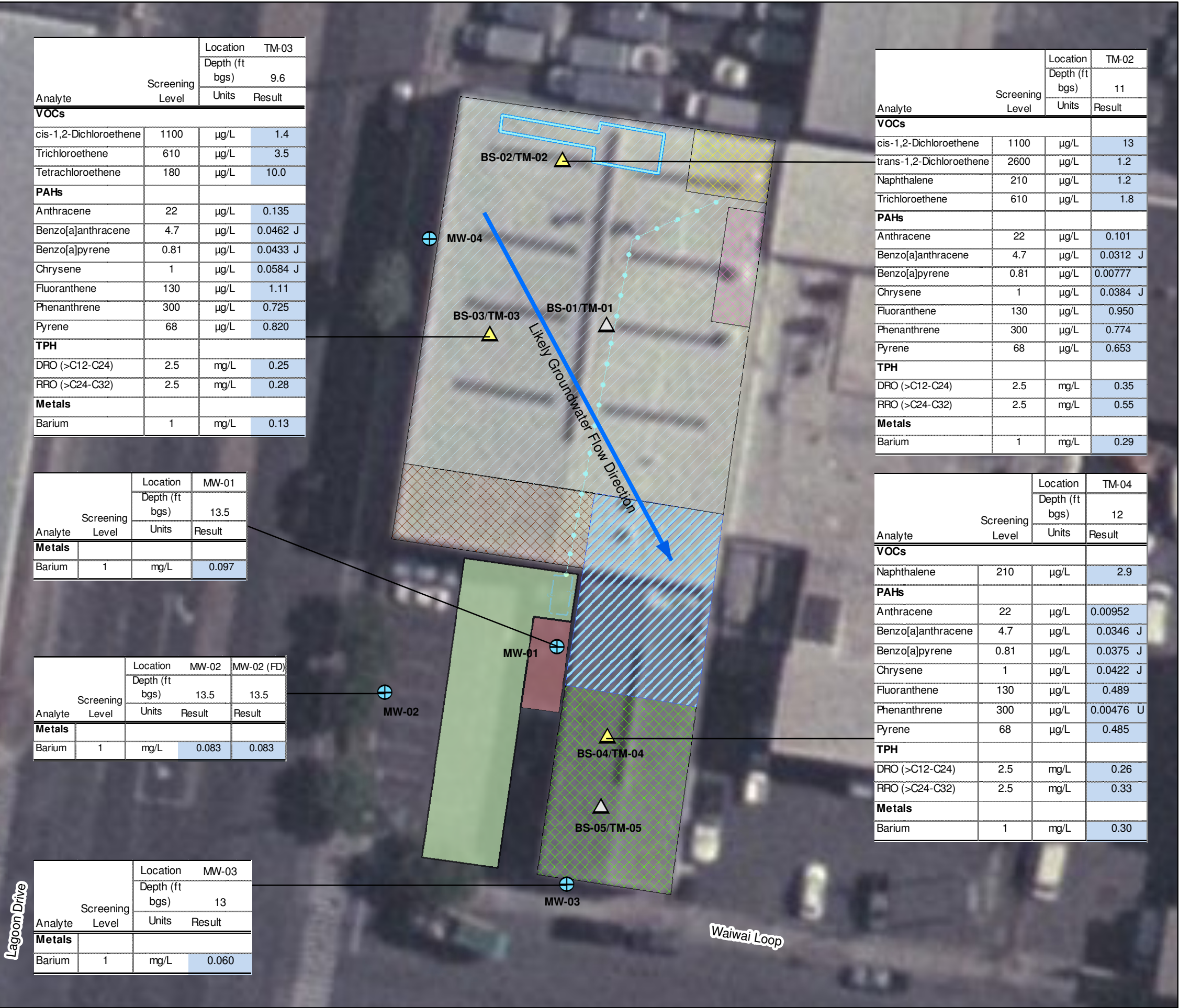
Figure 4 Detected Target Analytes in Groundwater and Geophysical Survey Coverage for Locating UST Phase II ESA 515 Lagoon Drive, Parcel 15 Honolulu, Oahu, Hawaii
