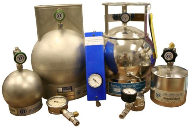
Soil Vapor Sampling Equipment - Summa Canisters, Flow Controllers, and Pressure Gauges
