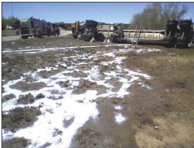
Figure 4. Irregular and disconnected spill patterns on soil made by a release of milk. This might also mimic vertical patterns for subsurface releases of liquids.
